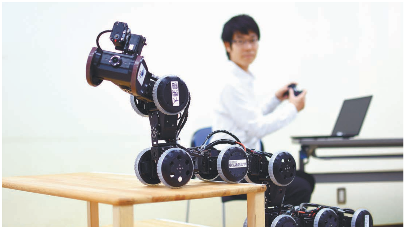
An older version of the snake-shaped robot, capable of climbing fairways and scale meter-high barriers. UEC
